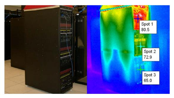
Figure 3) High density server being tested at increasing CPU utilizations.
