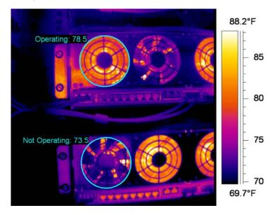
Figure 2) Server cooling fans are shown. The top fan is operating normally, while the bottom fan has failed.
