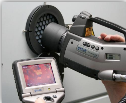
Figures 8a & 8b) Safety around electrical equipment is the #1 consideration during infrared surveying. Some of the options: 8a shows an IRISS infrared window installed in electrical cabinet 5 . The thermographer safely holds an infrared camera up against a viewing port or window to see inside the switchgear. These windows can be custom fit to any data center equipment. 8b) Thermographer wearing proper personal protective equipment (PPE) inspecting a battery bank during a full battery discharge test.
